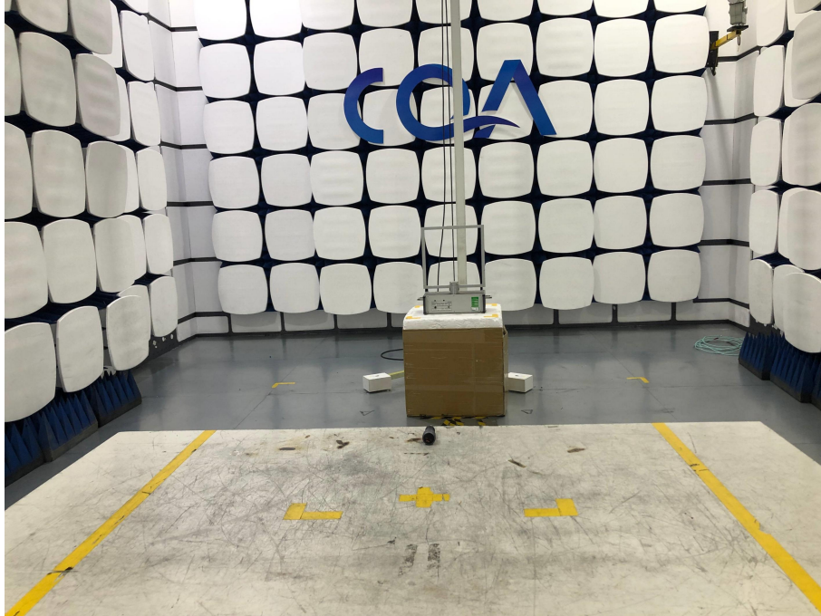
Radiated emission Test Setup-1(9kHz~30MHz)
