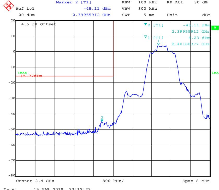
**Band Edge, Right Side**
