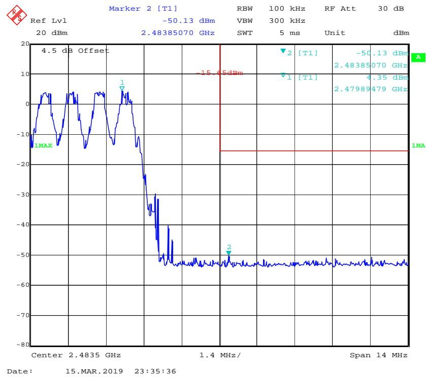
*EDR Mode ( $\pi/4$ -DQPSK):***Band Edge, Left Side**
