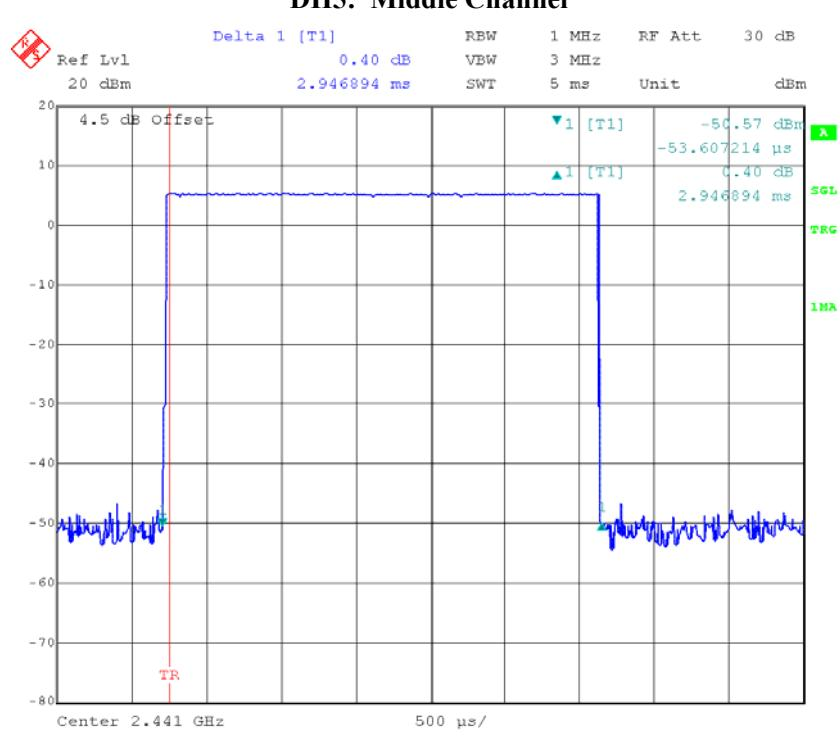
*EDR Mode ( $\pi/4$ -DQPSK):***2DH1: Middle Channel**
