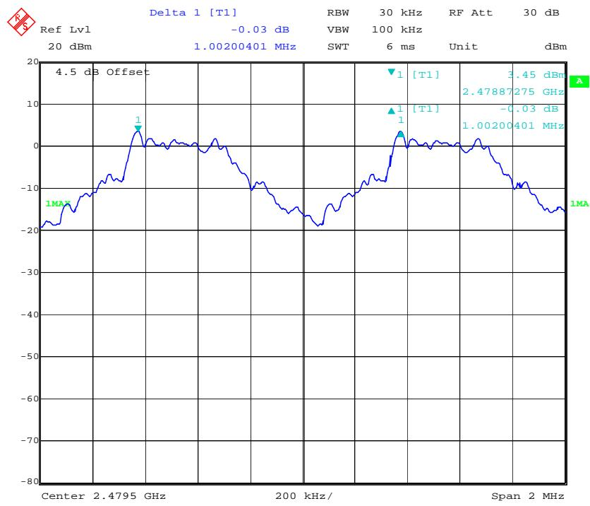
*EDR Mode ( $\pi/4$ -DQPSK):***Low Channel**
