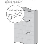
\*Insert anchors into wall.
