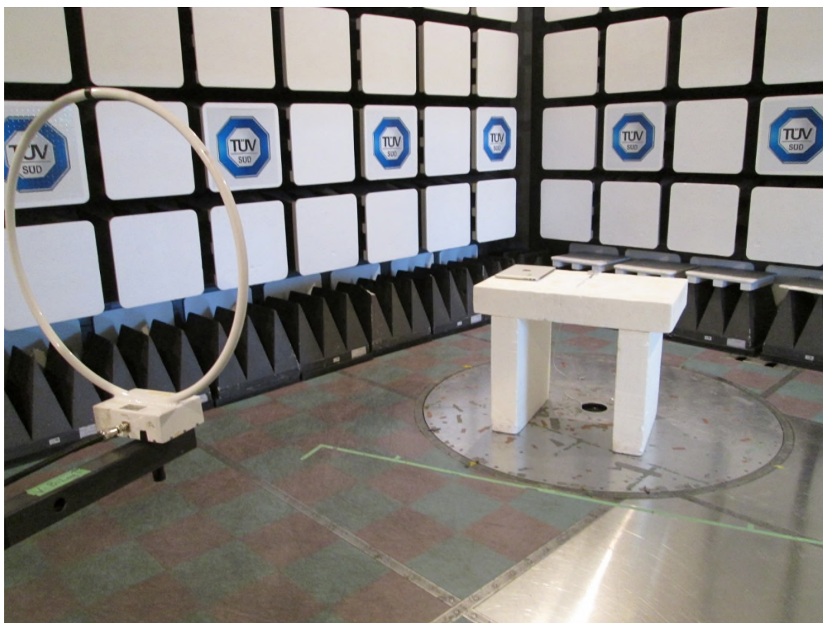
Test setup photo 1 Radiated measurements, 9 kHz – 30 MHz
