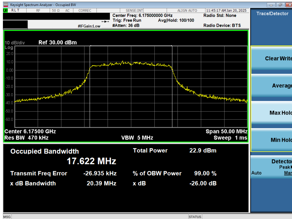
Plot 7-16. 26dB Bandwidth Plot MIMO ANT2 (20MHz 802.11a (UNII Band 5) – Ch. 45) – SP
