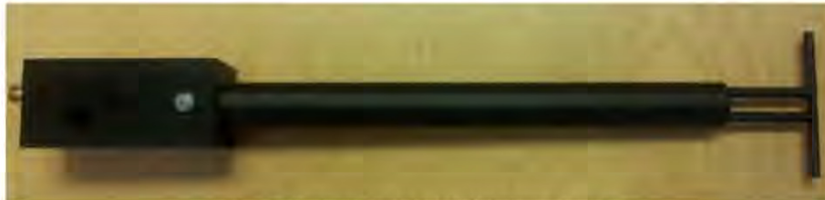
Figure 1 – MVG COMOSAR Validation Dipole
