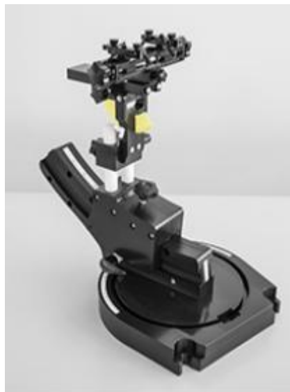
Device holder supplied by SPEAG
