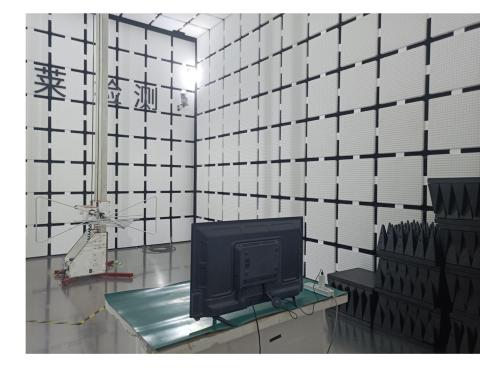
Radiated Emissions Test Setup Below 1G
