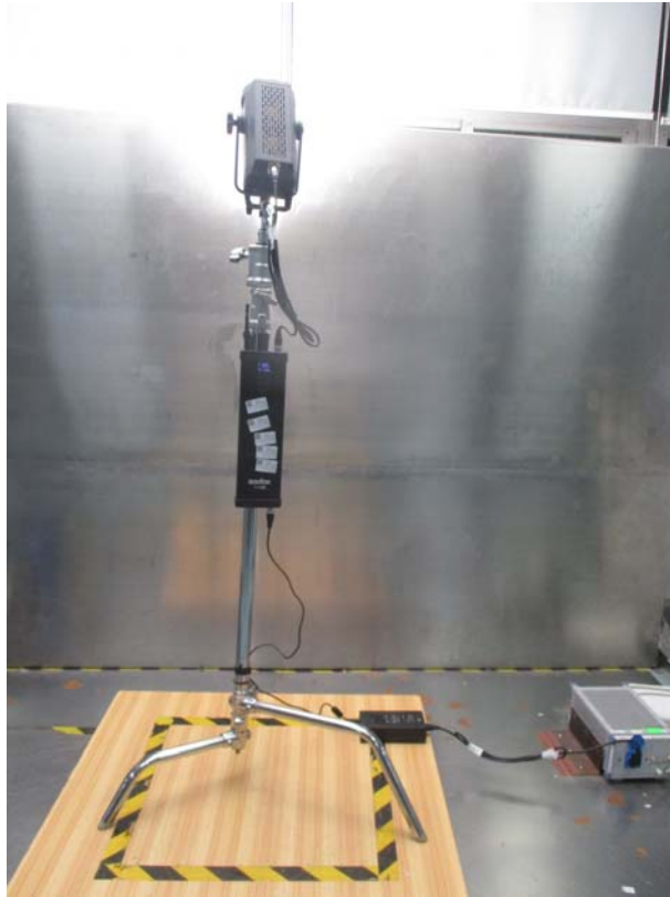
Conducted Emissions Side – VL300 View
