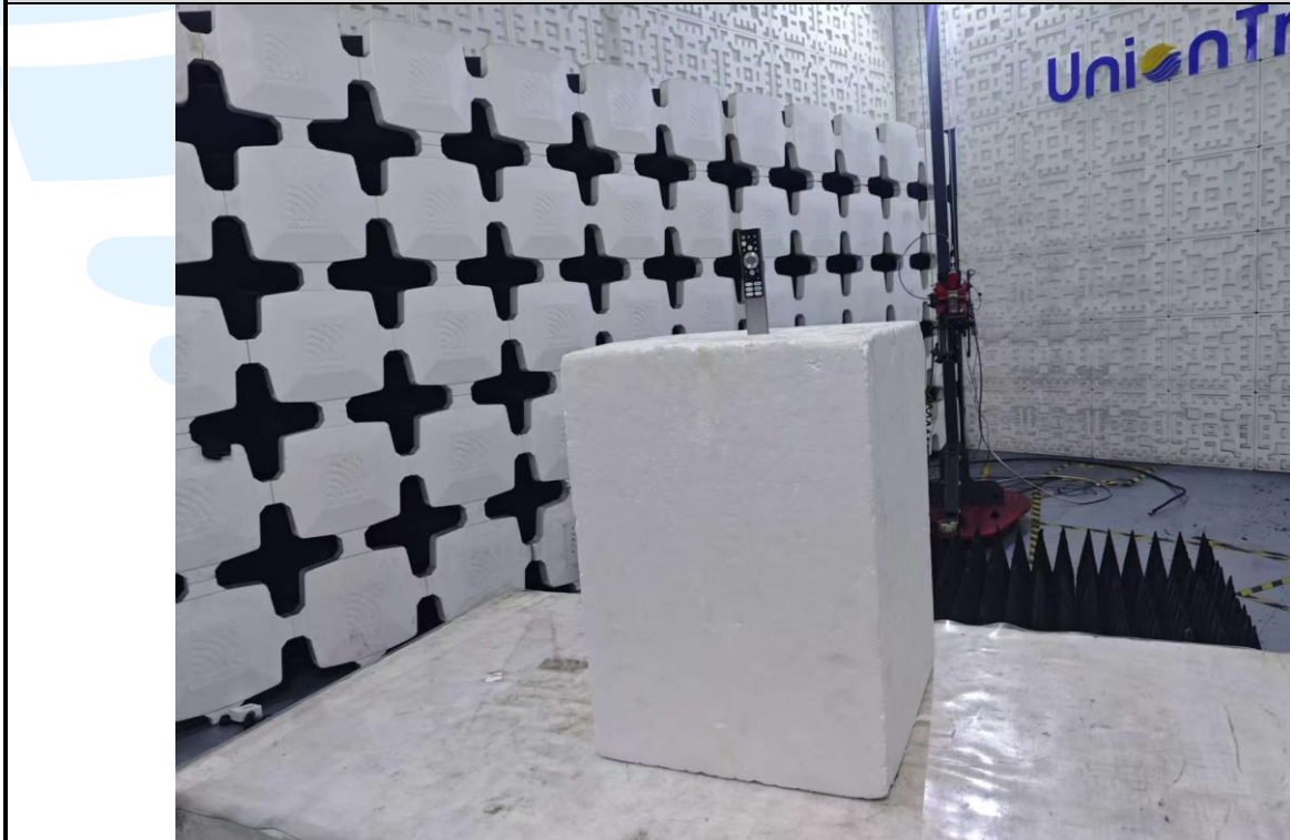
Radiated emission Test Setup (Above 1 GHz)
