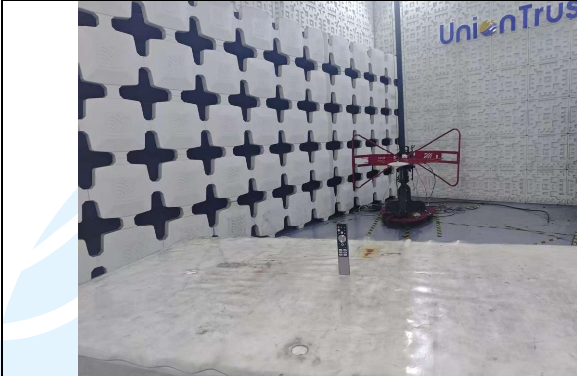
Radiated emission Test Setup (30 MHz~1 GHz)
