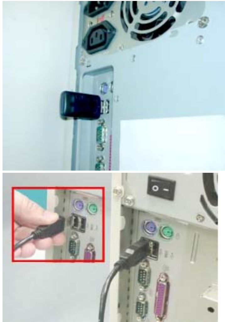
Figure 3-1: Plug the Bluetooth USB Adapter into USB port on desktop PC
