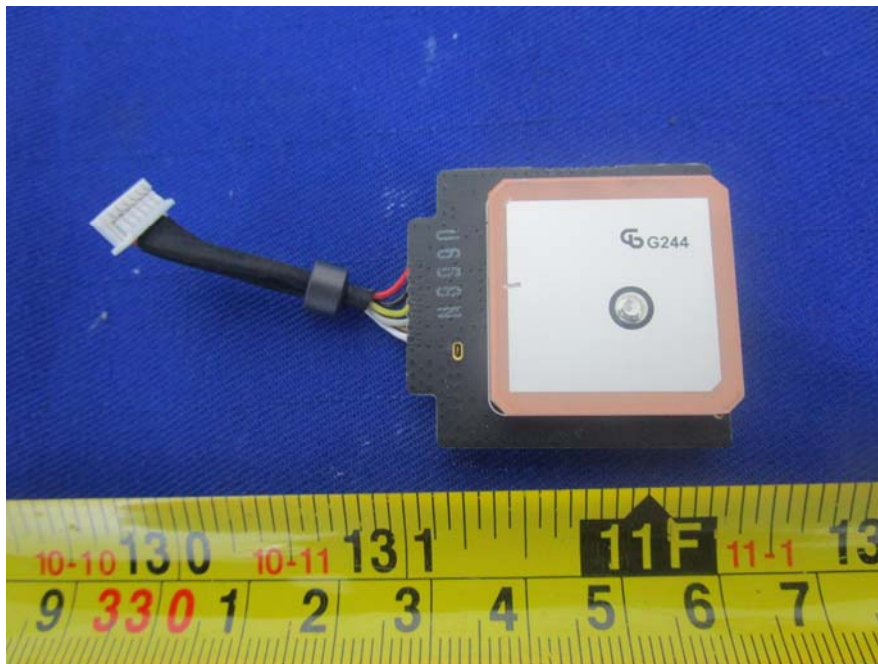
EUT –GPS Module Bottom&Antenna View
