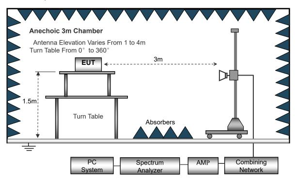
Frequency: 9kHz-30MHz Frequency: 30MHz-1GHz Frequency: Above 1GHz
