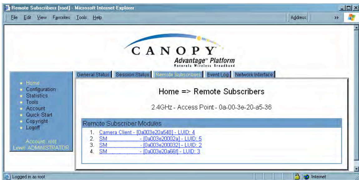
Figure 65: Remote Subscribers tab of AP, example
