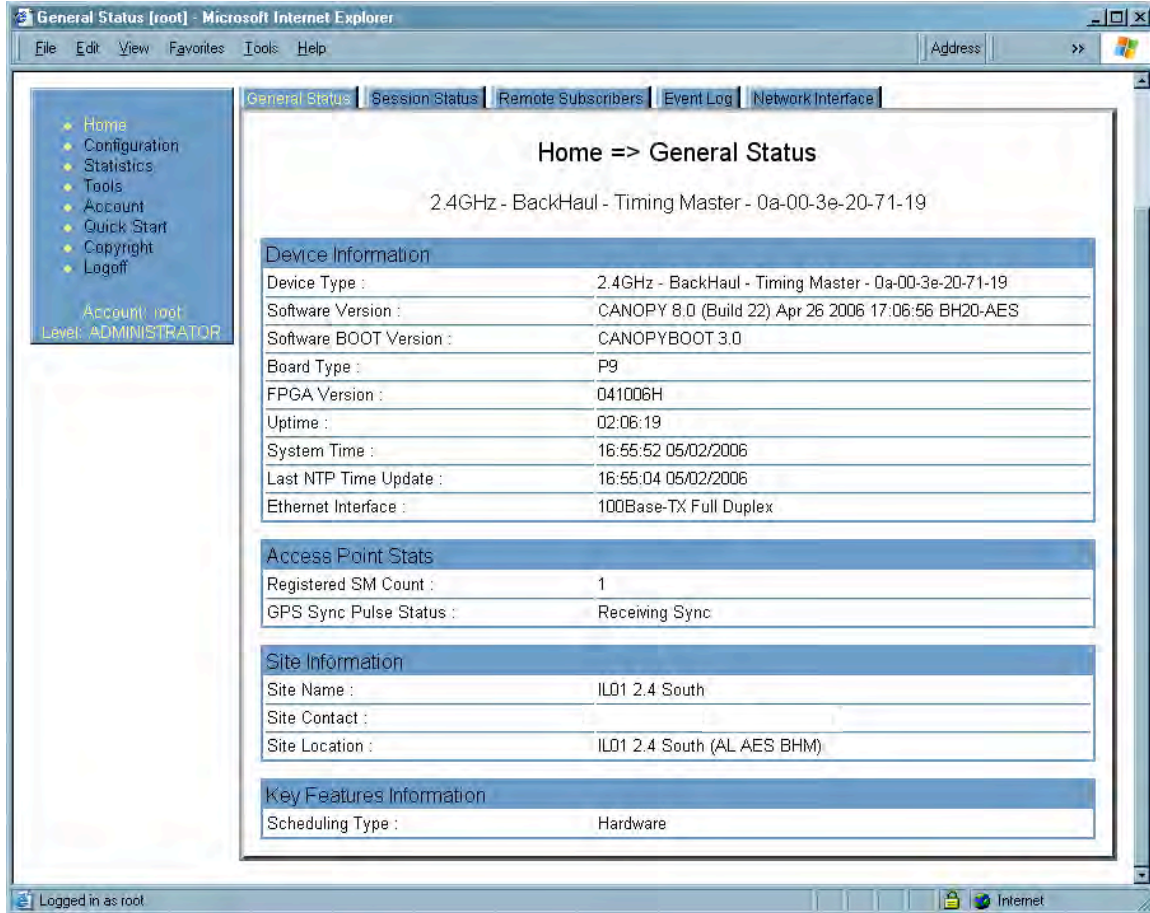
Figure 72: General Status tab of BHM, example
