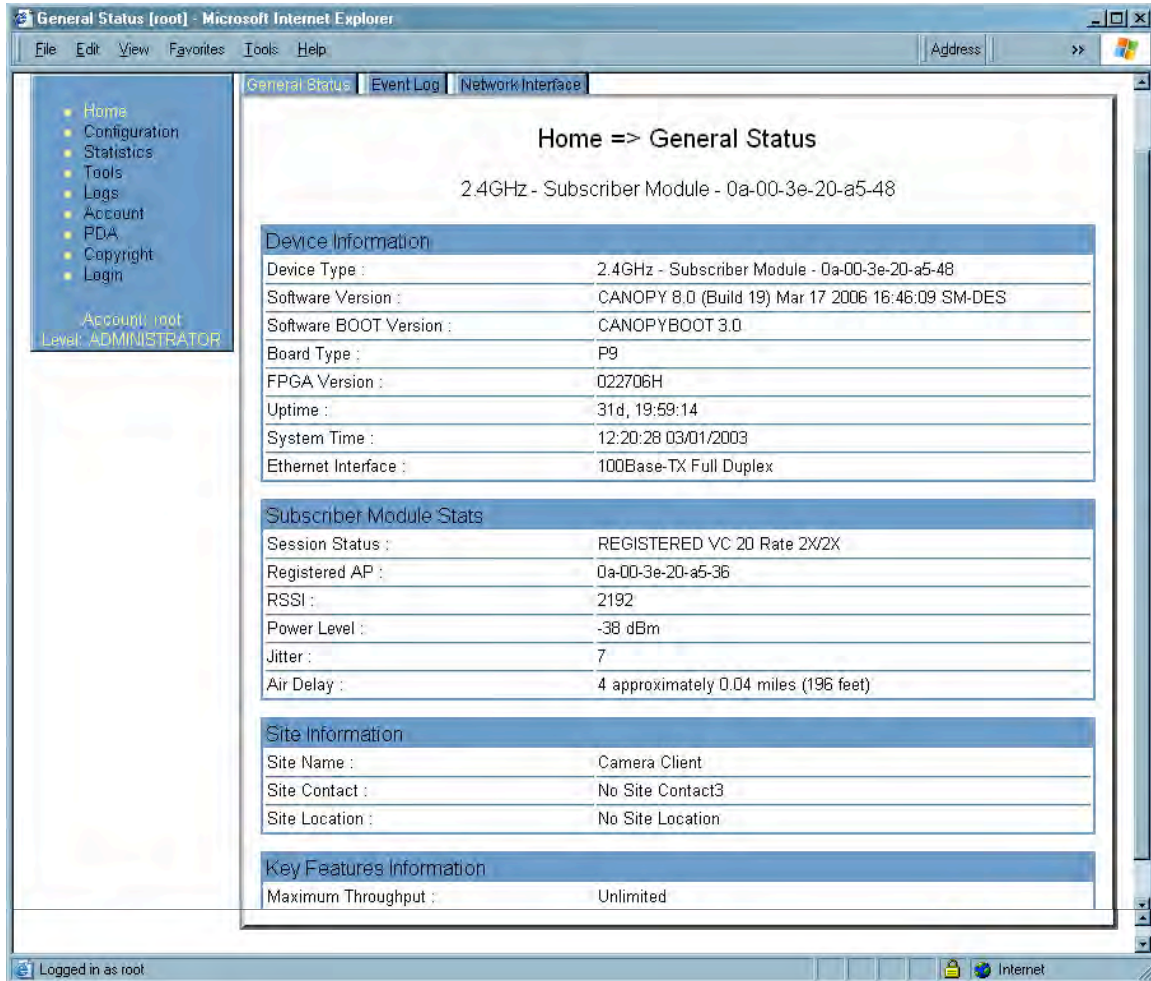
Figure 66: General Status tab of SM, example
