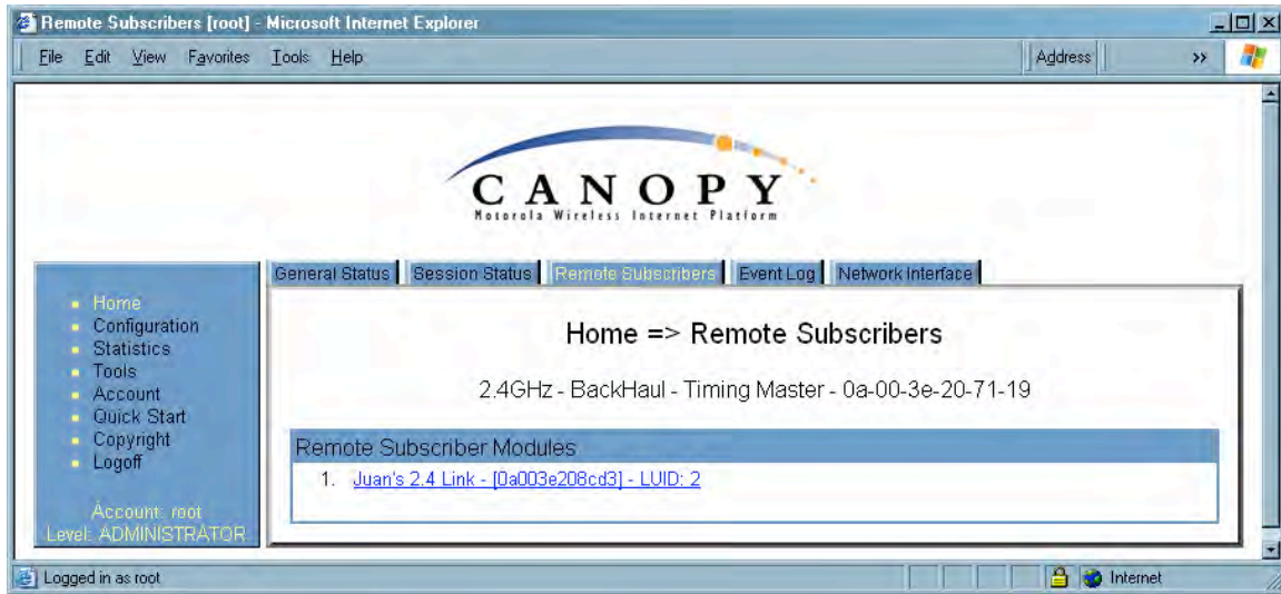
Figure 70: Remote Subscribers tab of BHM, example
