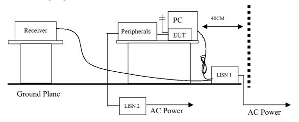
The EUT are connected to the main power through a line impedance stabilization network (LISN). This provides a 50 ohm/50uH coupling impedance for the measuring equipment. The peripheral devices are also connected to the main power through a LISN that provides a 50ohm/50uH coupling impedance with 50ohm termination.
