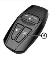
If the vehicle is locked when the DECK LID button is pressed, the doors will remain locked and the security system will still be armed.
