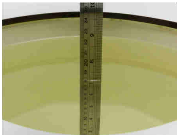
Fig 10.1 Photo of Liquid Height for Body SAR
