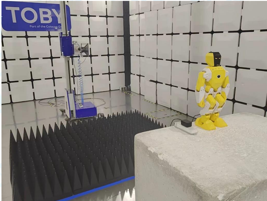
Photo of Setup for Conducted Emission
