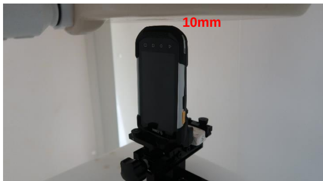
Bottom Side, Test Separation 10 mm
