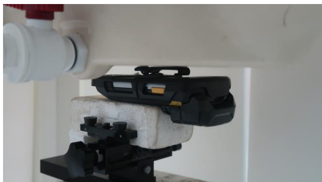
Front with Rigid Holster, Test Separation 0 mm
