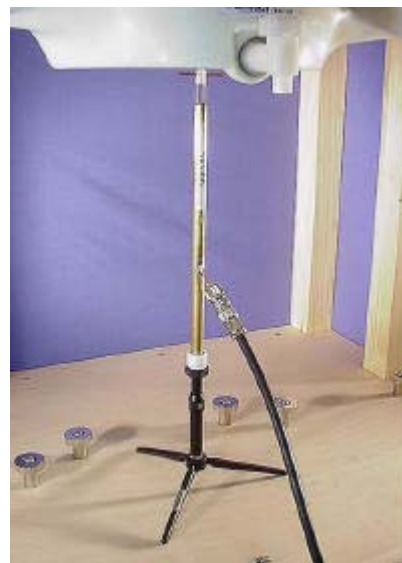
2450MHz Dipole Validation Setup
