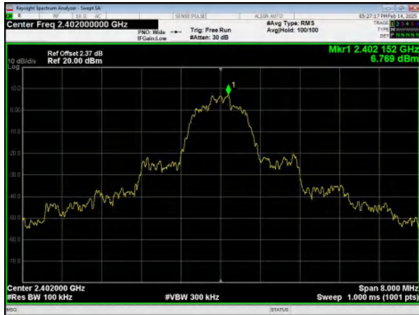
\pi/4 -DQPSK No-hopping Band edge-left side
