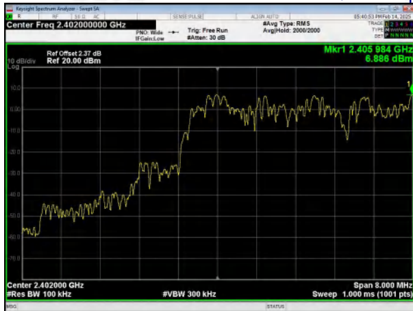
\pi/4 -DQPSK Hopping Band edge-left side
