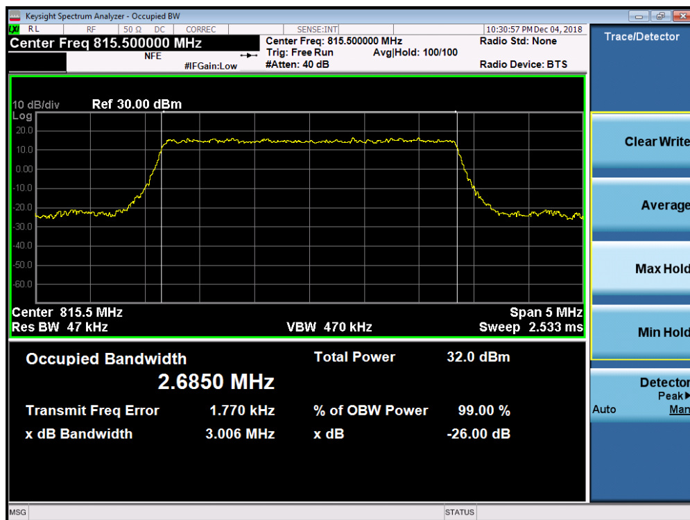
Plot 7-6. Occupied Bandwidth Plot (LTE Band 26, 3MHz QPSK – RB Size 15– Low Channel)
