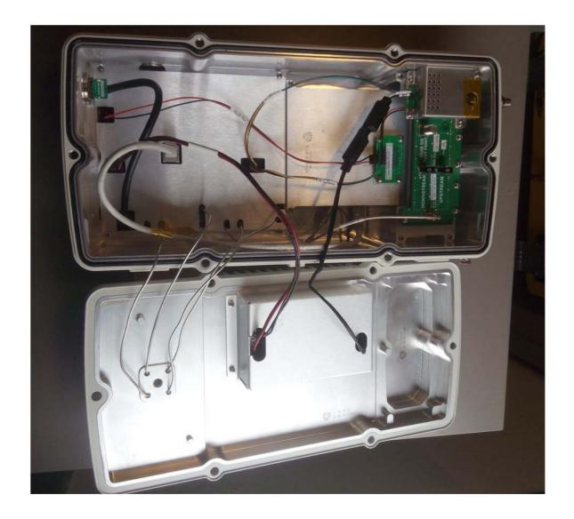
Photograph No.2 "AirStrand1300 2.6 GHz (B41)" base station internal view
