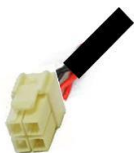
Figure 33: DC Power connector pre-assembled on converter
