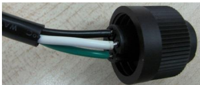
Figure 46: AC/DC converter wires assembled
