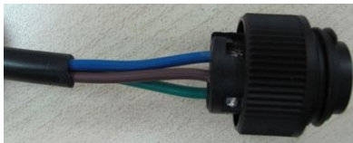
Figure 42: Power cable wires assembled
