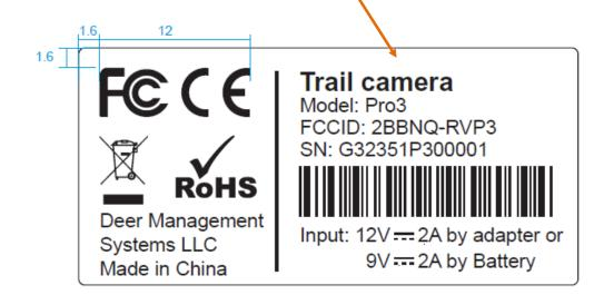
Size: 40x19mm, R0.5mm, tolerance:0~-0.1mm,
