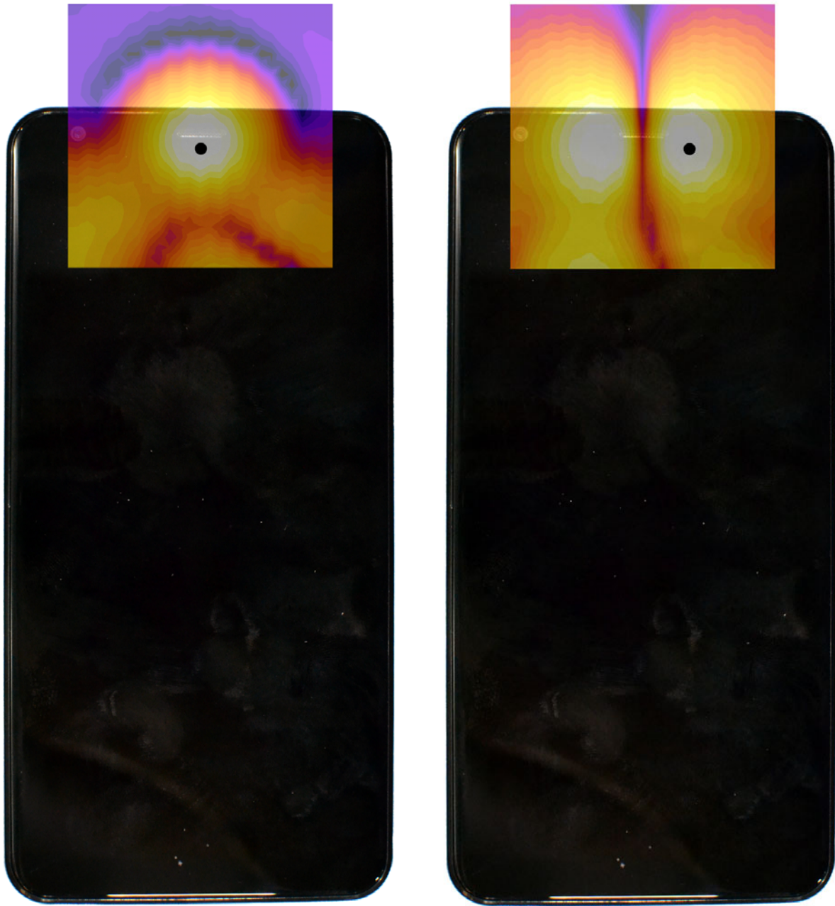
Figure 16-3 T-Coil Scan Overlay Magnetic Field Distributions
