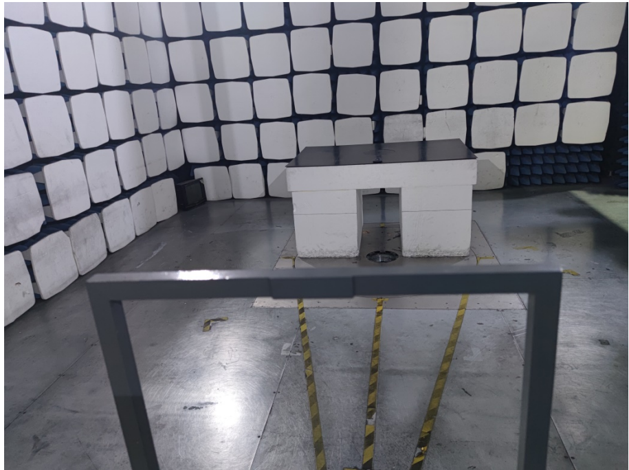
Radiation Emission Test Setup (Below 30MHz)
