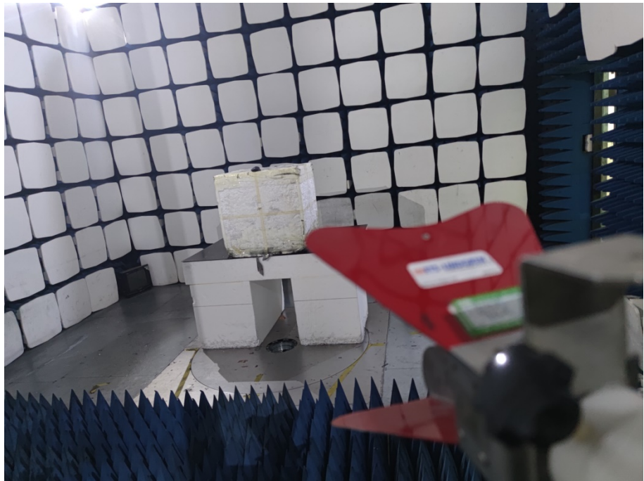
Radiation Emission Test Setup (1GHz to 18GHz)
