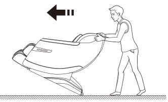
Warning: The rear moving wheels of the massage chair are only suitable for short-distance and slow movement. For long-distance transportation, please use other auxiliary moving tools to move this massage chair!
