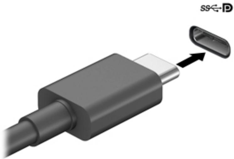
2. Connect the other end of the cable to the external DisplayPort device.
