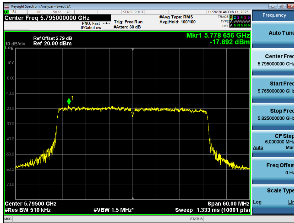
PSD NVNT ac40 5795MHz Ant1
