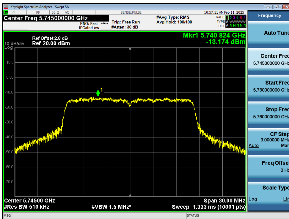
PSD NVNT a 5745MHz Ant1
