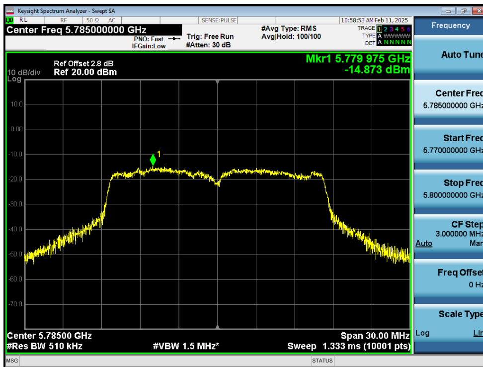
PSD NVNT a 5785MHz Ant1
