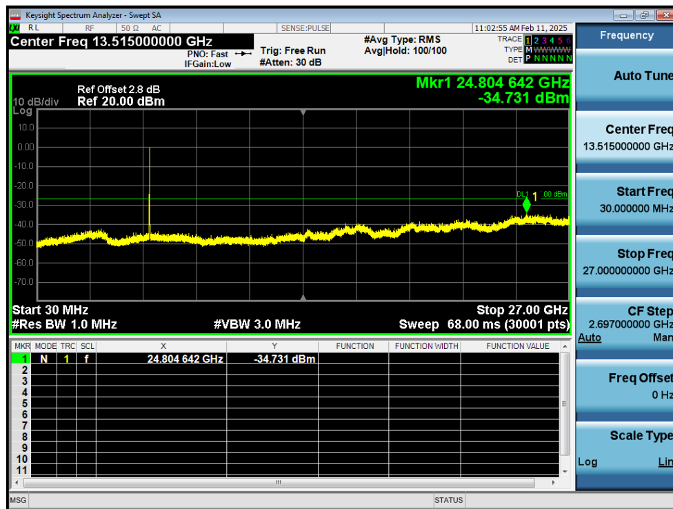
Tx. Spurious NVNT n20 5745MHz Ant1 Emission
