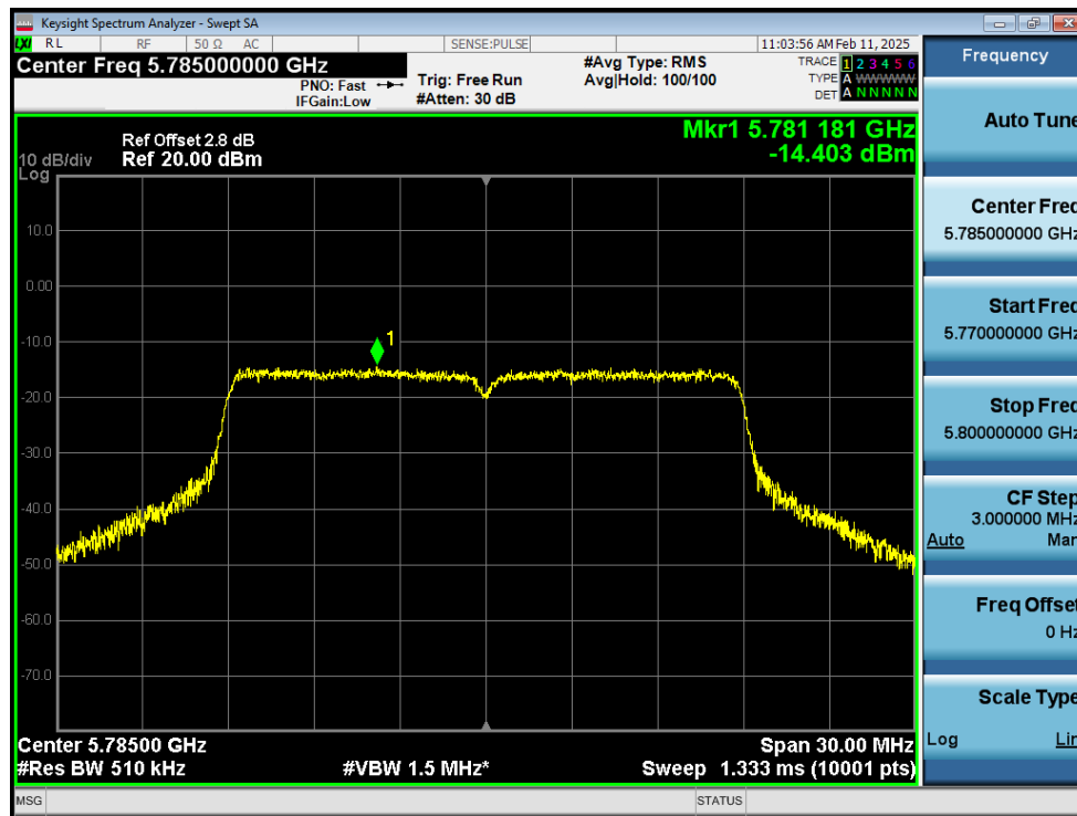
PSD NVNT n20 5785MHz Ant1
