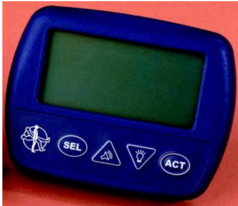
Figure 5: Personal Pump Communicator (PPC)
