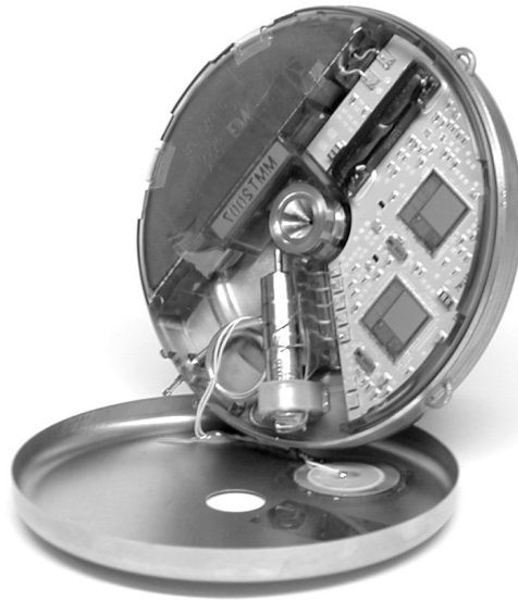
Figure 3: Interior of the Implantable Insulin Pump
