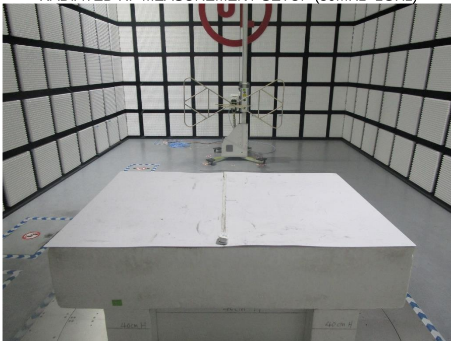
RADIATED RF MEASUREMENT SETUP (Below 30MHz)
