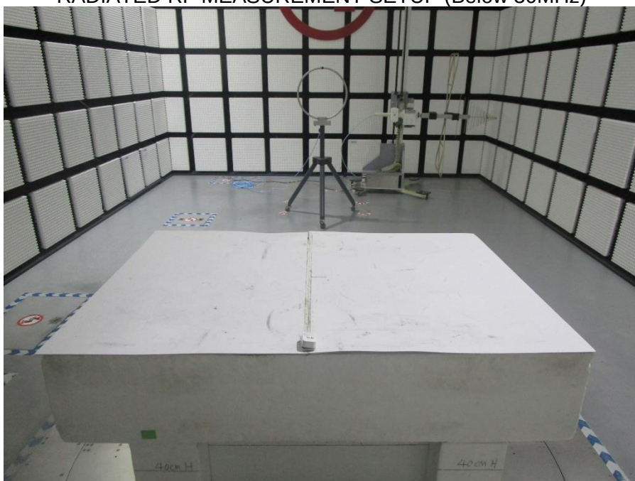
RADIATED RF MEASUREMENT SETUP (Below 30MHz)
