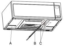
A. Bottom Plate B. Grease filter and Charcoal Filter
