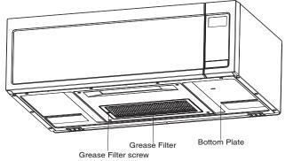
Hold the left side of the Grease filter, swing it to the right 2. position, and remove it from the slotted area.
