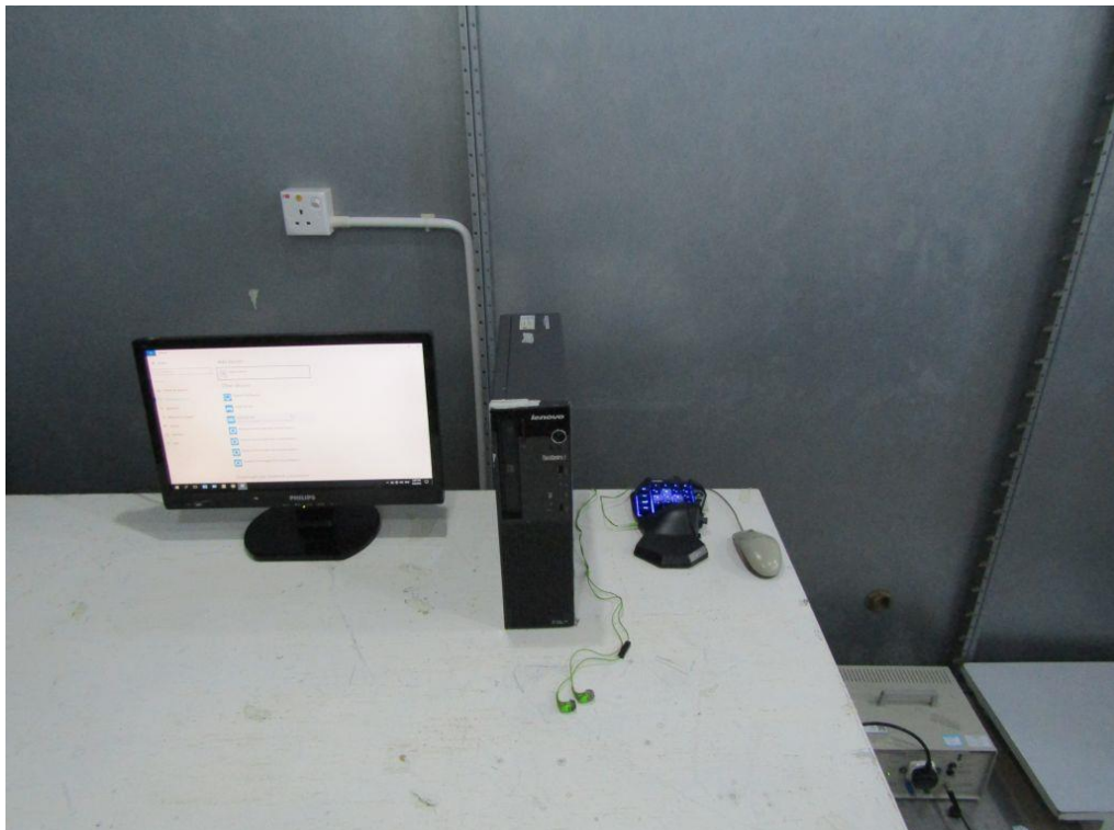
Measurement of Conducted Emission Test Set Up
