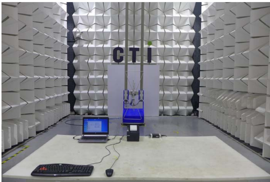
Radiated emission Test Setup
