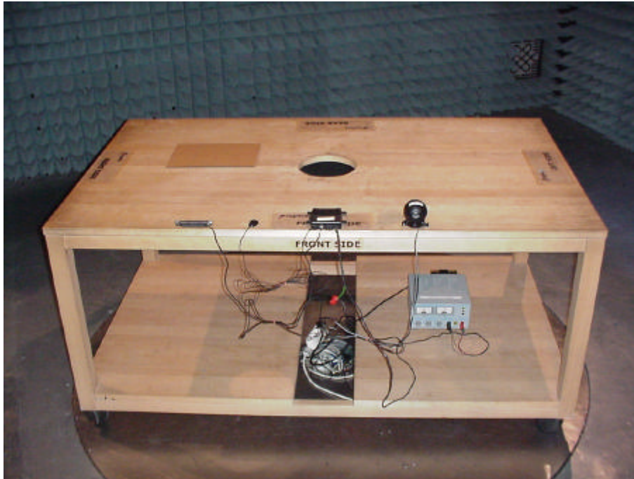
Picture 1 : Setup for radiated emission test
