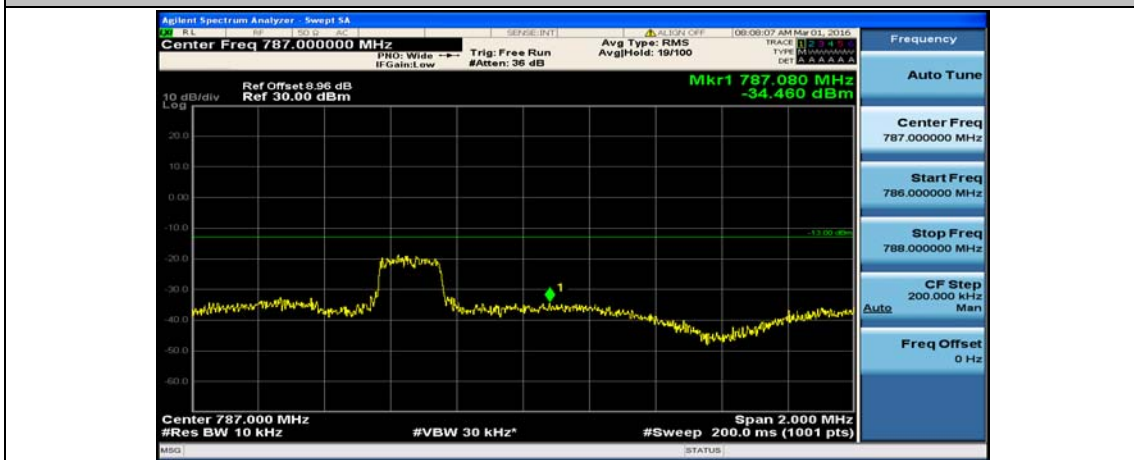
(Channel Bandwidth: 5 MHz)_HCH_QPSK_1RB#12
