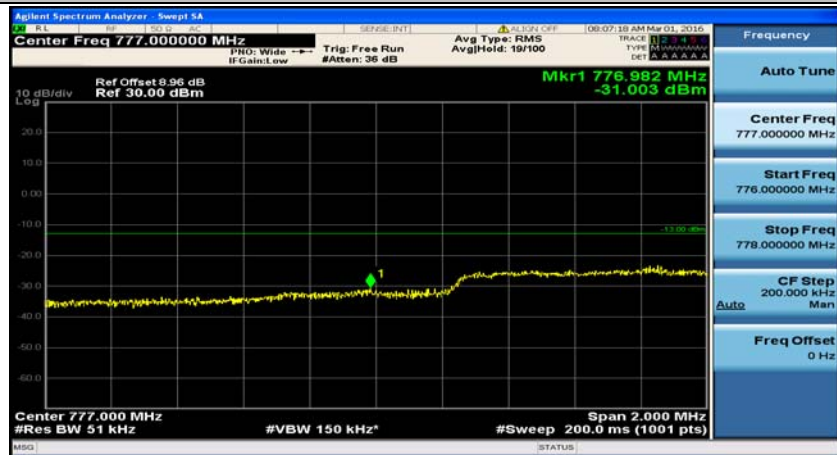
(Channel Bandwidth: 5 MHz)_LCH_QPSK_25RB#0
