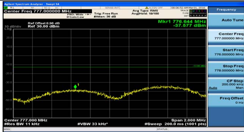
(Channel Bandwidth: 5 MHz)_LCH_16QAM_1RB#24
