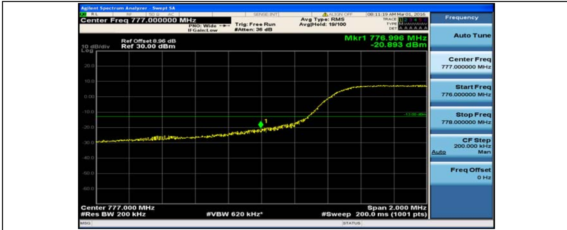
Channel Bandwidth: 10 MHz_HCH_16QAM_1RB#0
