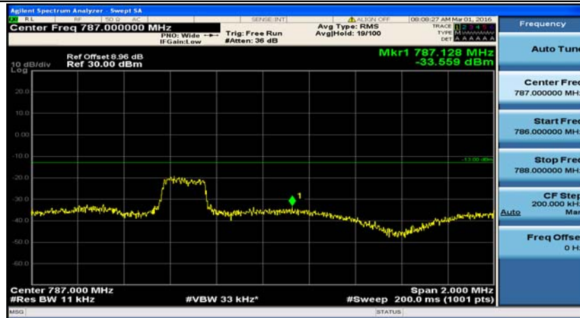
(Channel Bandwidth: 5 MHz)_HCH_16QAM_1RB#12
