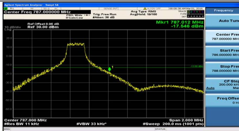
(Channel Bandwidth: 5 MHz)_HCH_16QAM_12RB#0
