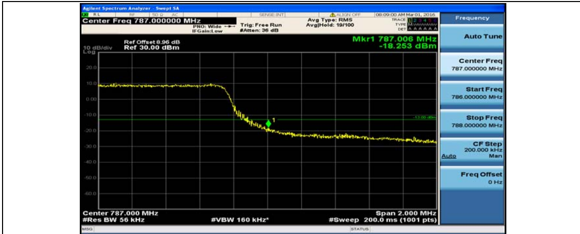
(Channel Bandwidth: 5 MHz)_HCH_QPSK_25RB#0
