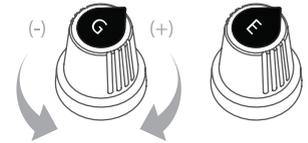
Each 1/4 inch port has its own **GAIN** and **ECHO** knobs that can be adjusted independently.
