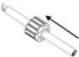
Figure 18: Insert Gland Nut
