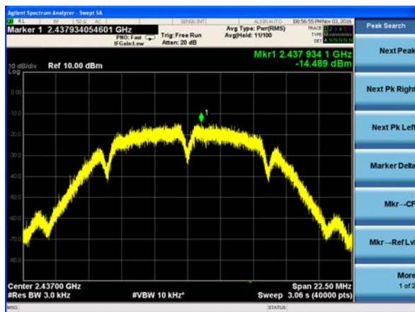
(802.11b) PSD plot on channel 6
