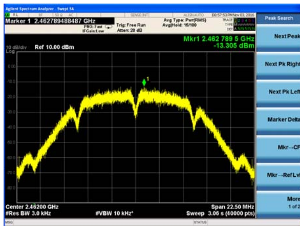
(802.11b) PSD plot on channel 11
