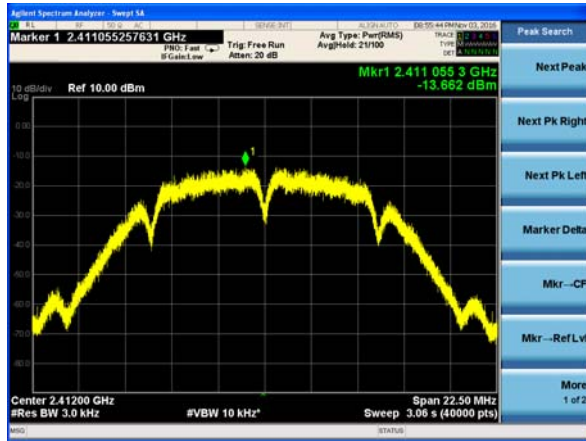
(802.11b) PSD plot on channel 6
