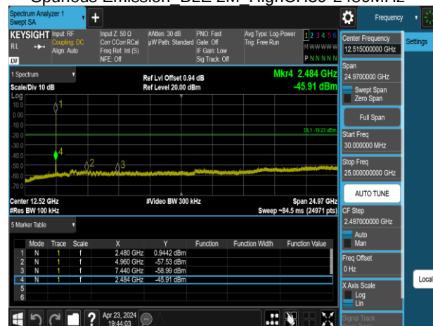
Spurious Emission BLE 2M HighCH39-2480MHz
