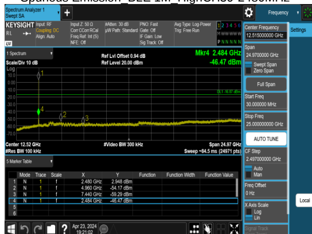
Spurious Emission BLE 1M HighCH39-2480MHz
