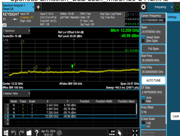
Spurious Emission BLE 125k HighCH39-2480MHz
