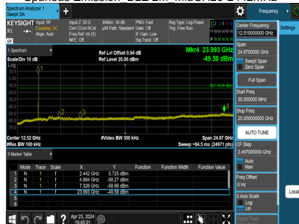
Spurious Emission BLE 2M HighCH39-2480MHz
