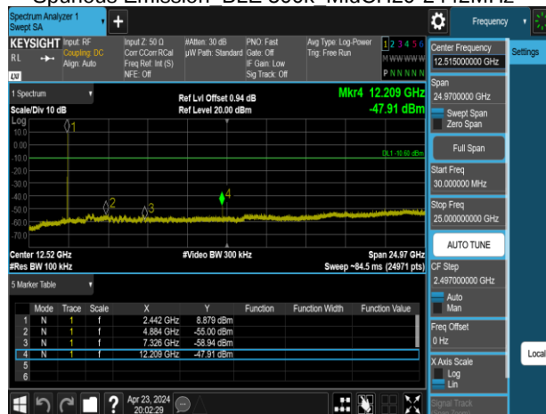
Spurious Emission BLE 500k HighCH39-2480MHz
