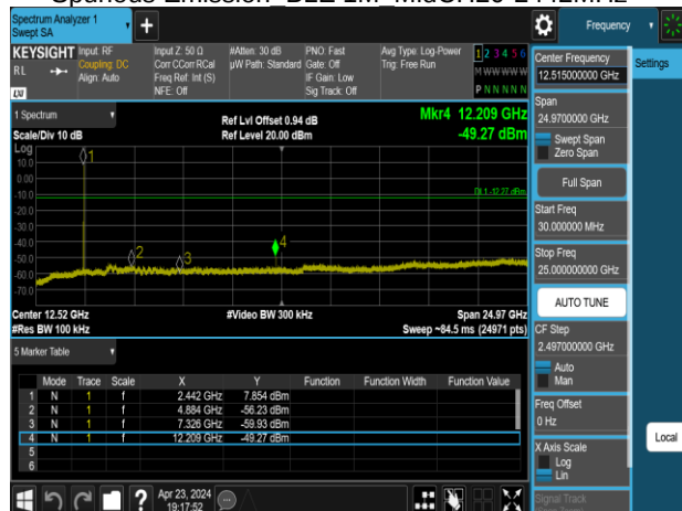
Spurious Emission BLE 1M HighCH39-2480MHz
