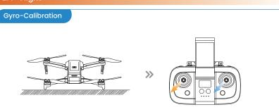
Make sure to place the drone on a level surface before calibrating the gyro. Simultaneously push the left joystick and the right joystick to the bottom left corner to calibrate the gyro. The indicator lights on the drone will blink, then turn solid, which indicates that the calibration is completed.
