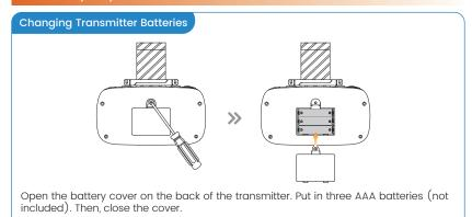
\*Low Battery Signal: The indicator lights on the transmitter flash slowly.
