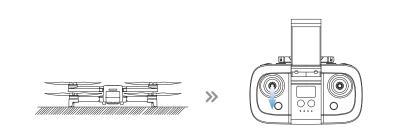
2 After the drone hits the ground, The drone indicator will keep on flashing. Please put the drone on a level surface again, and push the left joystick downward. The drone indicator then turn from flashing to solid, which indicates that you can use the drone now.
