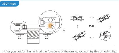
After you get familiar with all the functions of the drone, you can try this amazing flip mode. When the drone is at least 10 ft from the ground, press down on the button, then push the right joystick in any direction. The drone will perform a flip toward that direction
