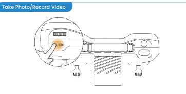
**Take Photo:** Short press the **(**) button on the transmitter to take a photo. The transmitter will beep once, signaling that a photo has been taken.
