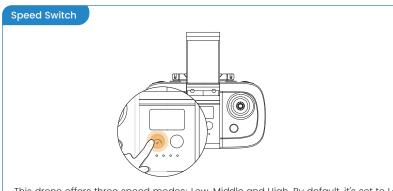
This drone offers three speed modes: Low, Middle and High. By default, it's set to Low speed.
