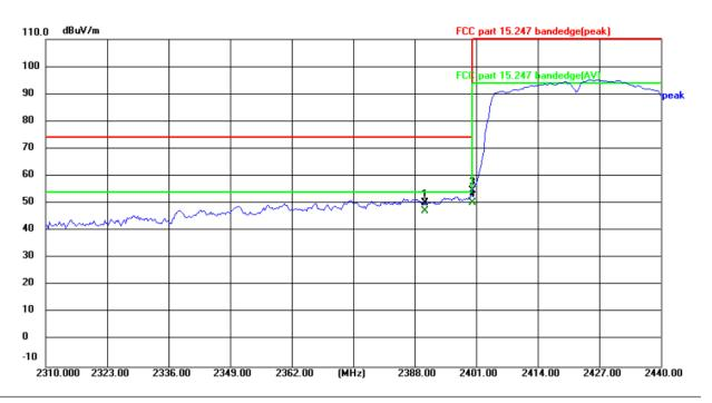
Site Polarization: Vertical Temperature: 24( $^{\circ}$ C) Limit: FCC part 15.247 bandedge(peak) Power: DC 3.7 V Humidity: 52 %
