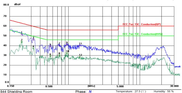
Site 844 Shielding Room Phase: N Temperature: 27.5 (°C)
