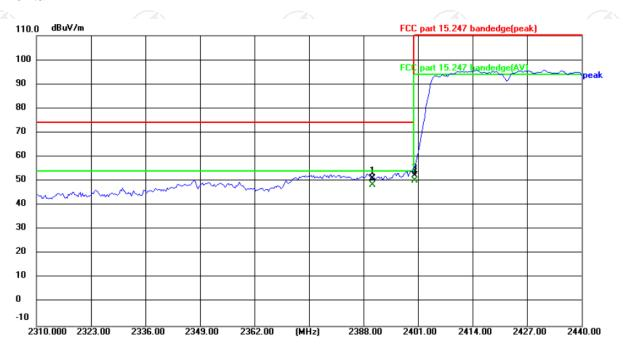
Site Polarization: Horizontal Temperature: 24( $^{\circ}$ ) Limit: FCC part 15.247 bandedge(peak) Power: DC 3.7 V Humidity: 52 %
