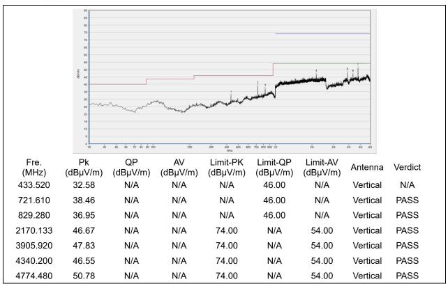
(433.92MHz, Antenna Vertical, 30MHz to 5GHz)
