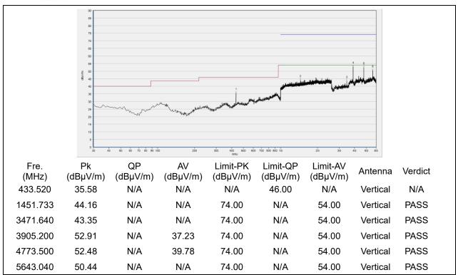
(433.92MHz, Antenna Vertical, 30MHz to 5GHz)
