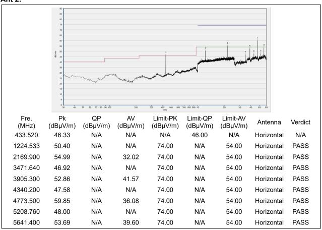
(433.92MHz, Antenna Horizontal, 30MHz to 5GHz)
