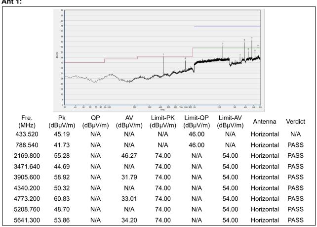
(433.92MHz, Antenna Horizontal, 30MHz to 5GHz)
