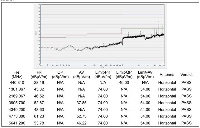
(433.92MHz, Antenna Horizontal, 30MHz to 5GHz)
