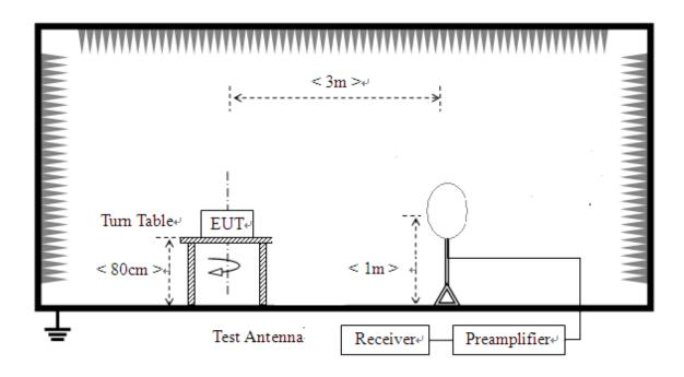
2) For radiated emissions from 30MHz to1GHz
