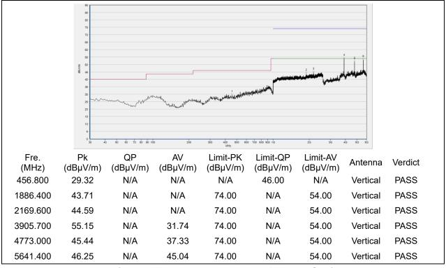
(433.92MHz, Antenna Vertical, 30MHz to 5GHz)
