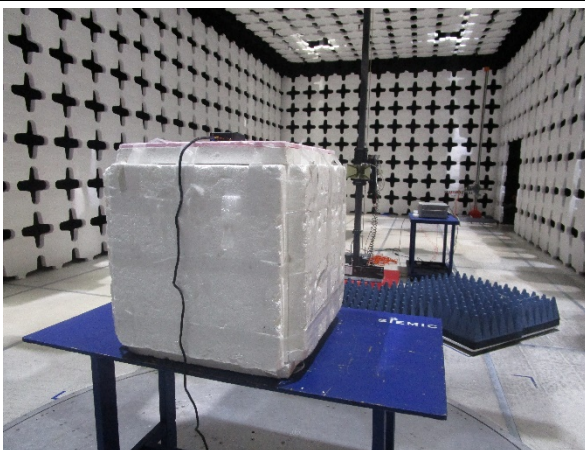
Radiated Emissions (>1GHz) – Rear View
