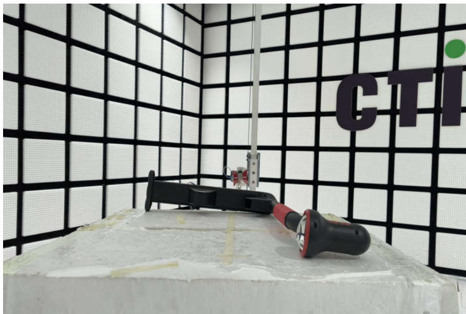
Radiated spurious emission Test Setup-3(Above 1GHz)
