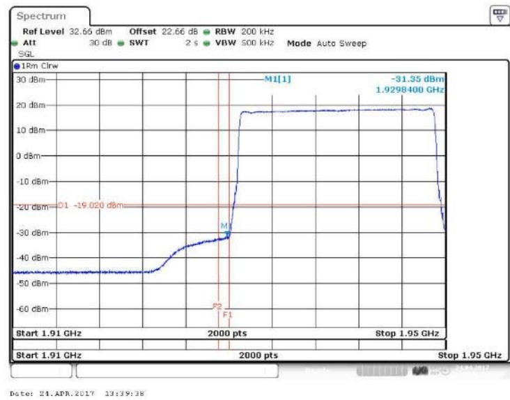
Figure 49 Spurious Emissions (Lower Band Edge) – 16QAM (1940.0 MHz) (20MHz Channel BW)
