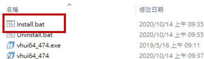
1. In the **VirtualHere** folder, double click **Install.bat** to install the software. Once it is completely installed, the program will launch automatically after you log into the computer.
