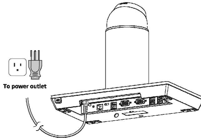
To use the premium docking station, firstly connect the AC adapter to the DC-in input and connect the other end to the power outlet. Always plug in the AC adapter first to enable the locking/unlocking function.
