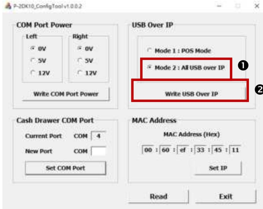
4. The default setting of the system is Mode 1: POS Mode. To change the default mode, select Mode 2: All USB over IP and tap on **Write USB over IP**.
