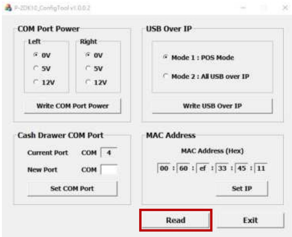
5. You can check the current setup condition by tapping on **Read**.
