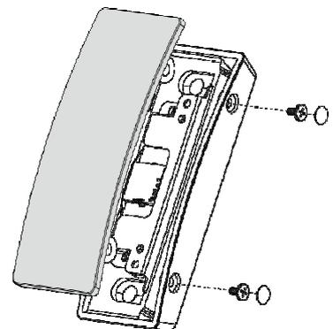
1. Remove the dummy cover first. Remove the rubber pads (x2) and screws (x2) to release the top cover of the MSR module.
