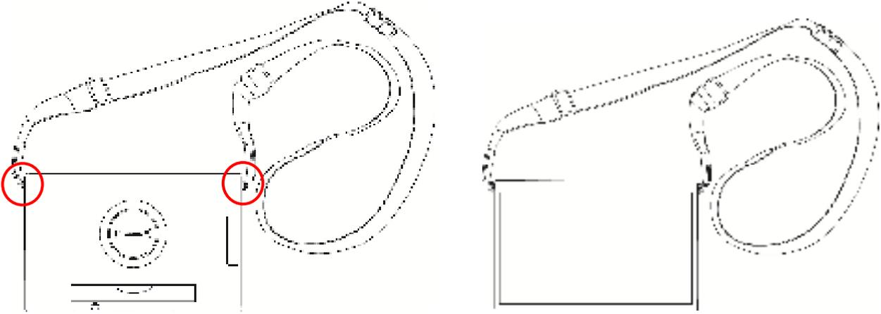
Align and attach the shoulder strap to the tablet as shown and fasten the screws (x2) to secure it.
