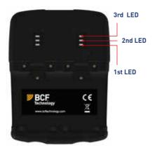
A fully discharged battery should be fully charged within 5.5 hours. While in a good condition, the battery run time will be 5 hours (assuming 50% idle time between scans).
