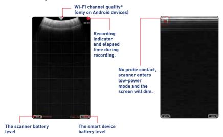
\*Change the channel in Wi-Fi settings. No indicator -clear channel in the 5GHz band. This is recommended state. White indicator-clear channel, but is on 2.4GHz band. It is more prone to interference. Orange/red indicator-channel with other networks or scanner. This is likely to cause interference issues.
