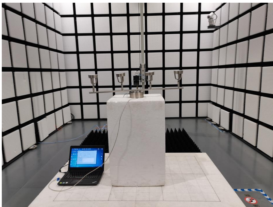
Fig. 3 Radiated emission setup photo(Above 1GHz)
