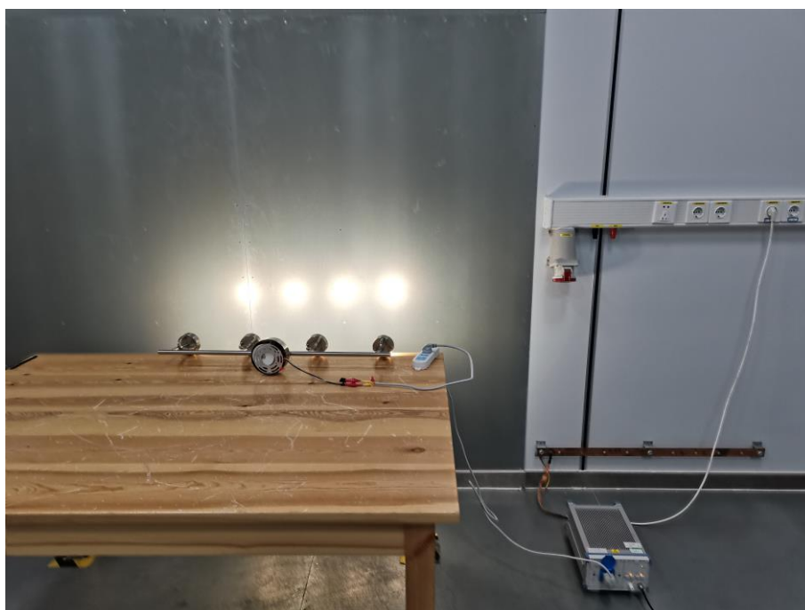
Fig. 4 Power line conducted emission setup photo
